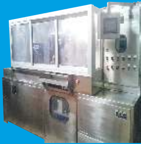
Horizontal Induction Hardening Machine with online Tempering
